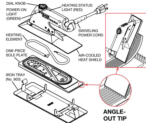
**Electronic Temperature Control:** Set a desired temperature on the dial between 240°F and 420°F and this iron will maintain that temperature continuously +/- 15°F. Initial overshoot and subsequent swings in temperature are reduced by this iron's highly sensitive thermistor and responsive digital control board. For your reference, ten temperature settings are marked on the dial corresponding to temperatures between 240°F and 420°F.
